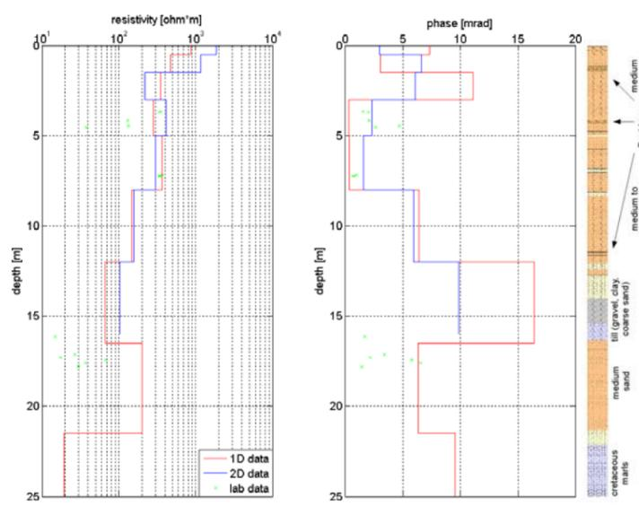
Fig.3: Comparison of 1D, 2D and lab data. Resistivity (left) and phase (right)
