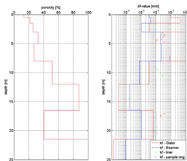
Fig.4: Porosity and kf estimates from 1D SIP data compared to lab kf data. SIP data derived from Fig.3
