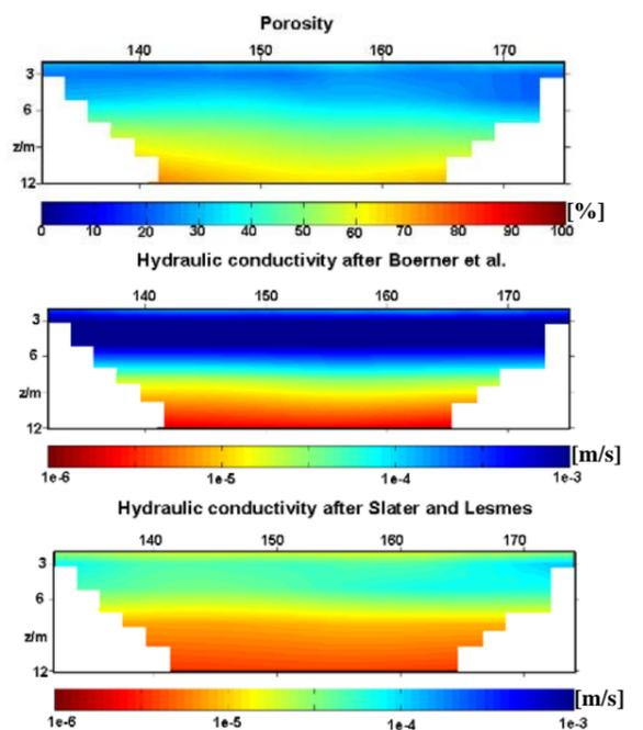
Fig.5: Porosity and kf estimates from SIP 2D data, derived from Fig.2
