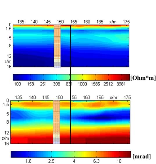
Fig.2: Inverted resistivity (top) and phase (bottom) model
