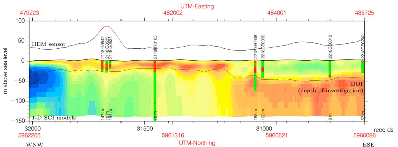
**Figure 4** Vertical resistivity section of 1-D SCI models along the cross-section in the pilot area Wanna (about 6800 m long). Lithology derived from nearby geologic borehole data is colour-coded: green colours indicate sand, red colours represent clay. For resistivity colour scale and location see Figure 1.
