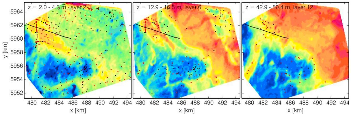
**Figure 3** Resistivity maps for three depth intervals from spatially constrained inversion (SCI) of HEM data for the pilot area Wanna. Black dots mark available geological borehole data in each depth interval. Red dots show where clay or silt layers of thickness > 2 m are present (independent of depth interval). The black line indicates the location of the cross-section displayed in Figure 4. For resistivity colour scale see Figure 1.
