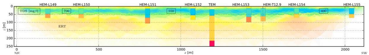
**Figure 2** Comparison of HEM/TEM resistivity-depth models along the ERT profile and estimated values of salinity in the aquifer along the cross-section in the pilot area Dollern. For resistivity colour scale and location see Figure 1.
