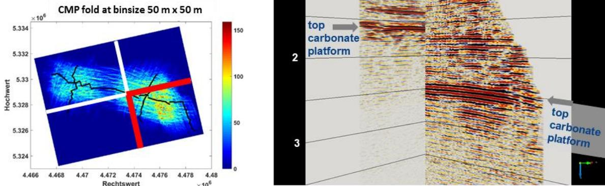
**Figure 3, left:** CMP fold of the MEMS receivers. Red lines show sections on the right. **Right:** CDP-Stack of Z- and H2-component face to face without time correction.
