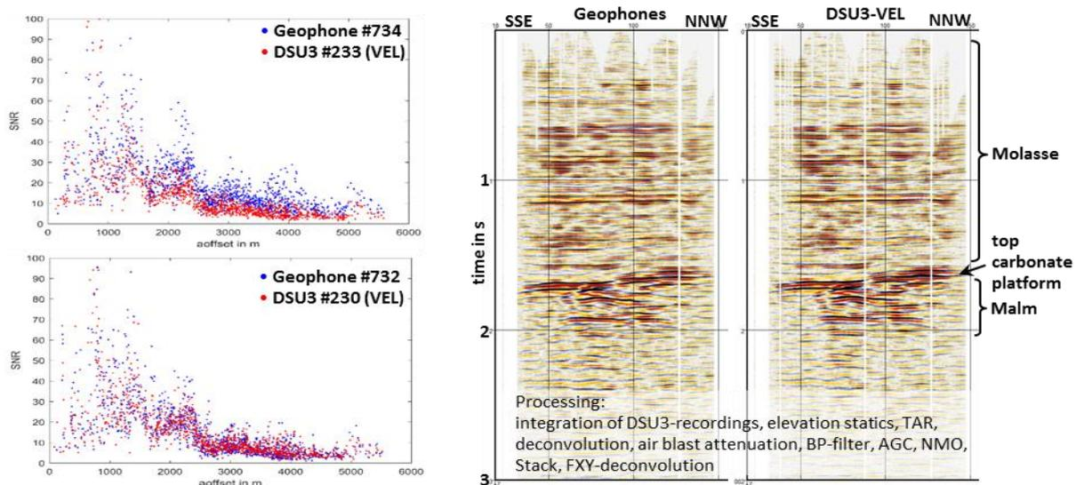
**Figure 2, left:** SNR of a geophone group (•) and a DSU3-sensor (•) recording at the same position. Two locations are shown, SNR was calculated using the RMS amplitude in a 150 ms long time window before and coincident with the P-Wave first break, respectively. **Right:** Stack of 51 geophone and DSU3 recordings, respectively. Processing steps are indicated in the figure.
