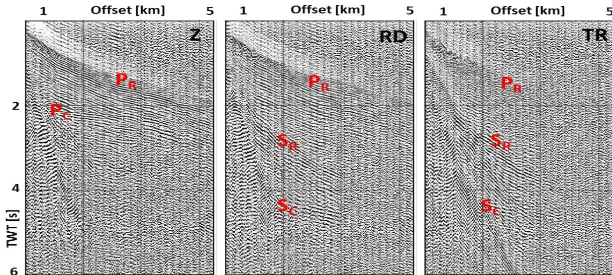
**Figure 5:** Single shot using the SHOVER technique. Shown are three components (Z vertical, RD radial, TR transversal). Traces are individual rotated according to receiver-source azimuth.  $P_r$  refracted P-waves,  $S_r$  refracted S-waves,  $P_c$  P-reflection and  $S_c$  S-reflection at the top of the carbonate platform.
