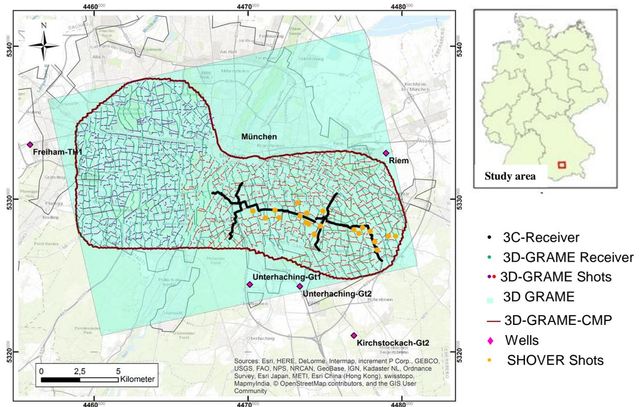
**Figure 1:** Map of the GRAME seismic survey in the southern part of Munich. Black lines mark positions of 3C MEMS receivers, that recorded regular shots from the 3D survey (red points) as well as 20 SHOVER shots (yellow points).
