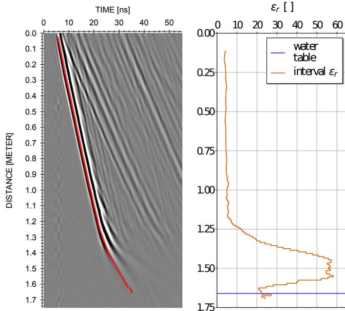
Fig. 2. Left: processed radargram of field data with a picked zero crossing phase (red) of the guided wave. Right: corresponding permittivities calculated from the travel-times in the intervals (orange), water table (blue).
