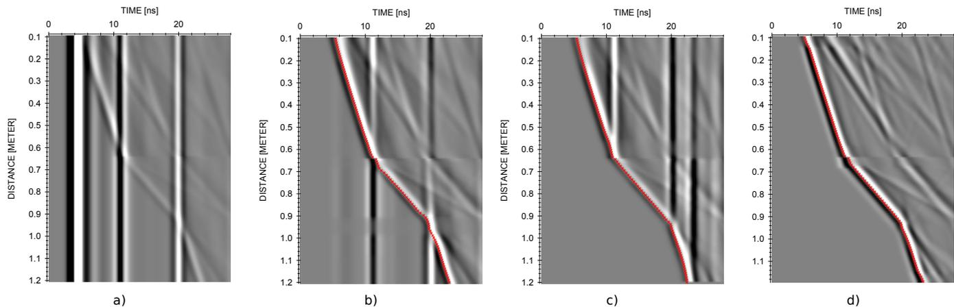
Fig. 6. Radargrams of the guided waves in layered media after applying different processing techniques, with the picks shown in red. a) raw radargram, b) background removal, c) subtracting the last trace, d) subtracting a moving average of 10 traces.
