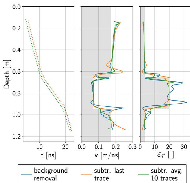
Fig. 7. Derived parameters from a simulation of guided waves in layered media, with the layer parameters depicted in gray. The waveguide was lowered with a 1 cm step, but the velocities and permittivities are calculated over a 4 cm interval.
