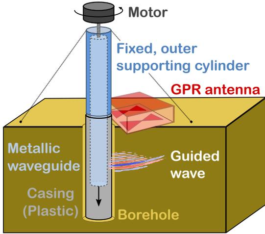
Fig. 1. Sketch of the guided GPR waves methodology.
