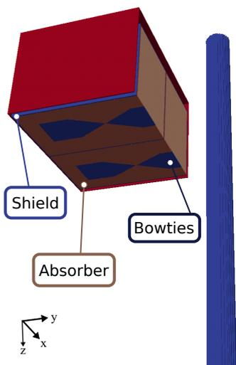
Fig. 3. View of the numerical 400 MHz antenna model, albeit truncated at two sides to allow to see the inside structures, and the metal cylindrical waveguide. The metallic case and bow-ties were modelled as perfect electric conductors.
