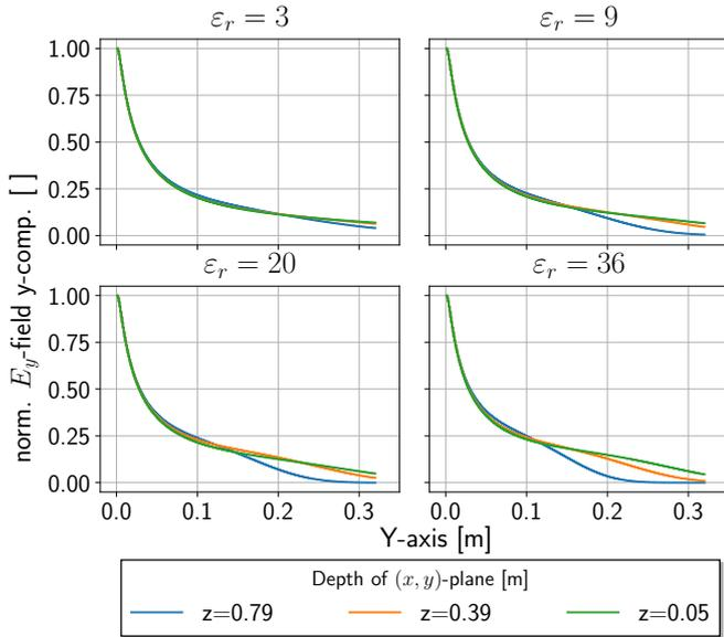
Fig. 5. Normalized electric field y-component amplitude with distance to the cylinder surface.
