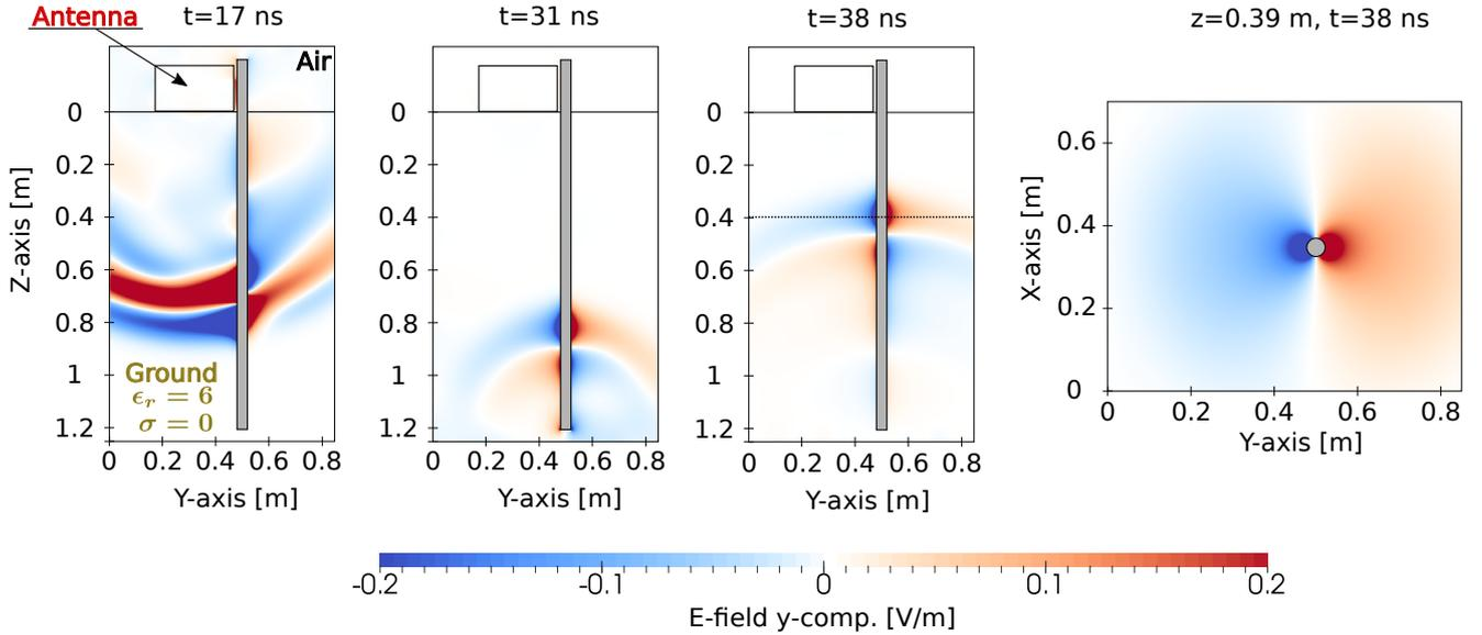
Fig. 4. Electric field distribution in the ground and around the metallic waveguide. The first three images show a vertical 2D slice through the middle of the antenna as well as the cylinder. The fourth image shows the horizontal distribution around the waveguide at  $z = 0.39$  m, indicated by the black dotted line in the third image.
