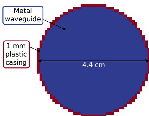
Fig. 8. Cross section of the metal cylinder with the 1 mm thick plastic coating.
