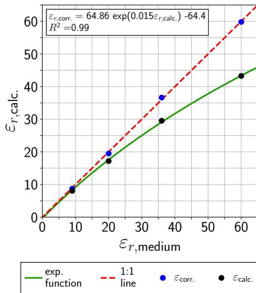
Fig. 9. Input and measured apparent permittivities, with the theoretical outcome lying on the red 1:1 line. The black dots depict the calculated permittivities in different media and under the influence of a plastic coating with a thickness of 1 mm. These are fitted with the green curves and corrected (blue dots) to the 1:1 line via the equation in the diagram.
