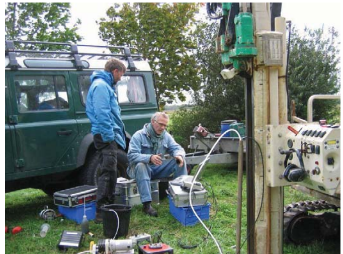
GEOPROBE® subsurface tests for a characterisation of underground structure and water sample collection conducted by colleagues from DTU and GEUS (© Paul Königer)
