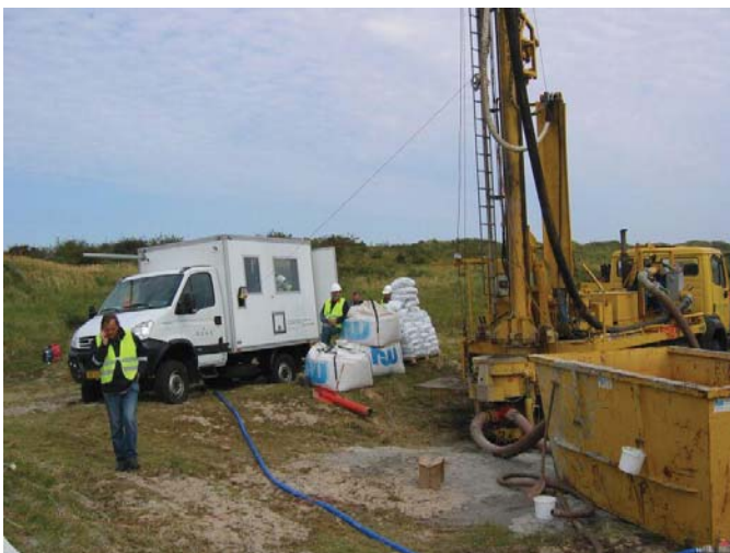
Borehole drilling and data logging in the Ostland catchment of the island of Borkum (© Paul Königer)
