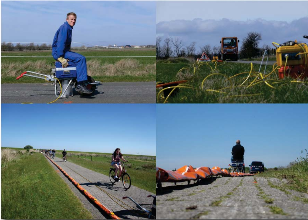
Figure 2: Impressions from seismic field surveys (clockwise): seismic vibrator source ELVIS mounted on a wheelbarrow. The coupling of the vibrations to the ground is improved by the weight of our colleague; vibroseis truck on the line and seismic recording unit in foreground; ELVIS and seismic streamer with geophones every meter; passers-by causing "noise" to our measurements (©Thomas Burschil & Helga Wiederhold)
