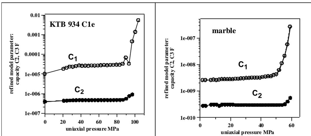
Fig. 5 Variation of the refined model parameters C1 and C2 as derived from the equivalent circuit model. Capacity C1 is the electrical parameter that correlates with the inner surface of the sample.
