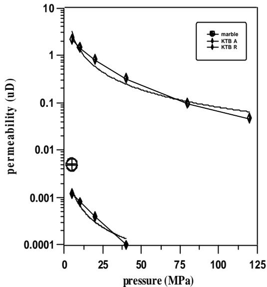
Fig. 1 Pressure dependence of the permeability of the marble and the KTB rock samples. The permeability was measured using a pressure transient technique with a pressure gradient of 5 MPa across the sample. The transport medium was Argon-gas. The confining (hydrostatic) pressure could be increased up to 300 MPa.
