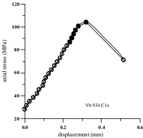
Fig. 3 Complete load displacement of a KTB amphibolite. The load was increased stepwise, because of measuring the complex electrical response for each step in pressure.
