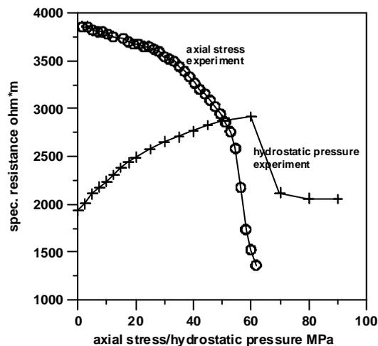
Fig. 2 Pressure dependence of the volume (bulk) resistivity of samples that were used in a hydrostatic (resistivity increase) and a triaxial pressure experiment (resistivity decrease).
