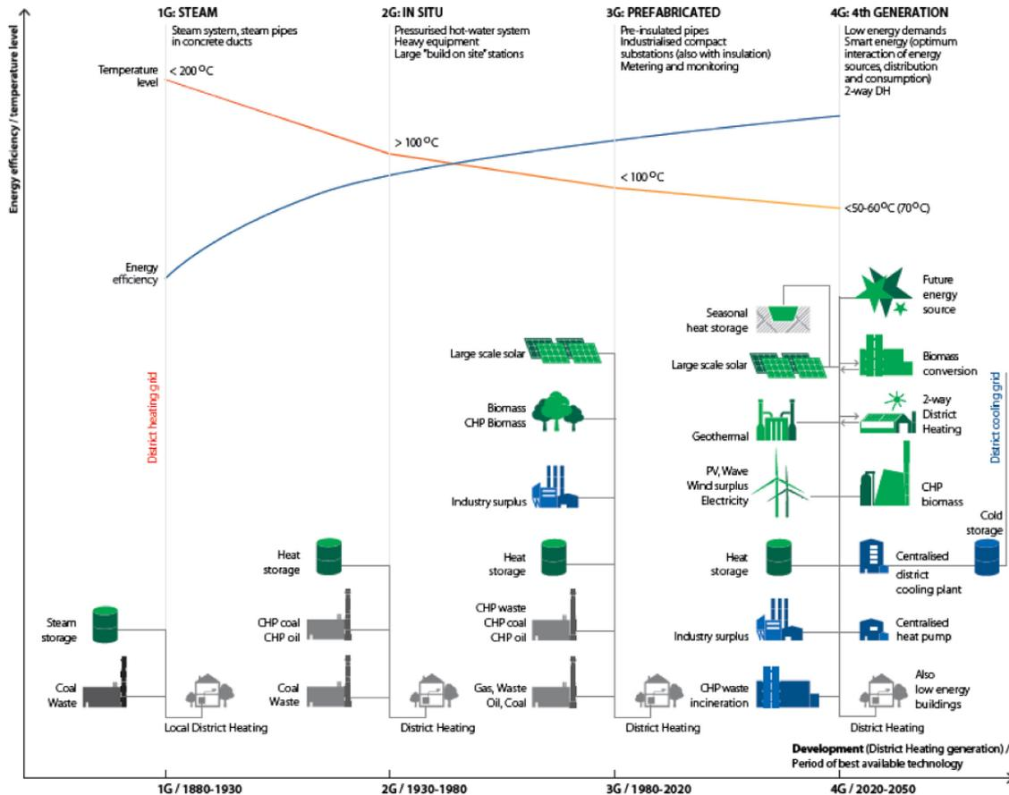
**Figure 1: Evolution of district heating and cooling networks with regard to temperature levels, energy efficiency and heat as well as cold sources (taken from Lund et al. 2014, p.9).**
